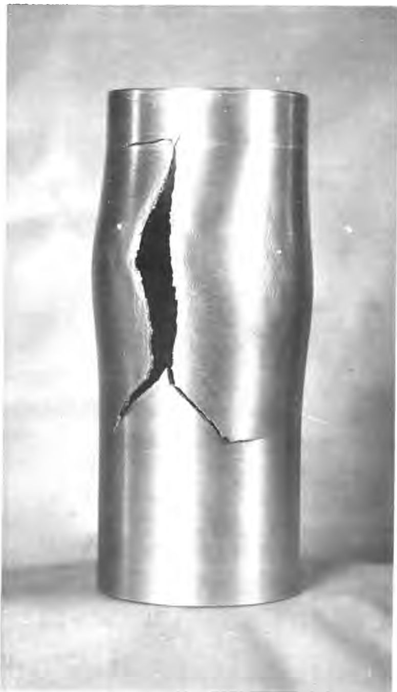
PHOTOGRAPH OF DRAWN HEXAGONAL SHRAPNEL CASE, AFTER RUPTURE BY INTERIOR HYDROSTATIC PRESSURE.
